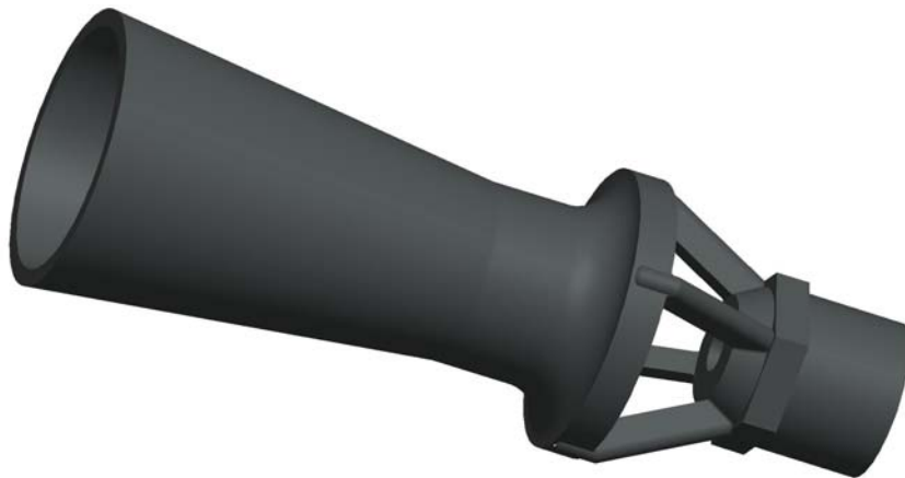
Fig. 4.6 CAD Model of a Hydraulic Mixing Nozzle
